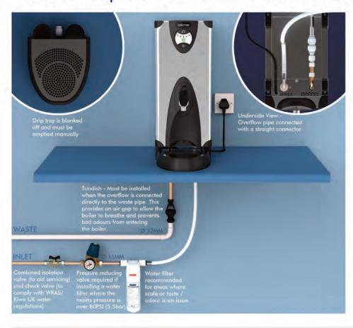
To help with planning the installation, a guide can be found in the Support section of our website. By selecting typical options to suit the particular location, a suggested configuration is displayed. Supplementary fittings and accessories are also shown for consideration.
